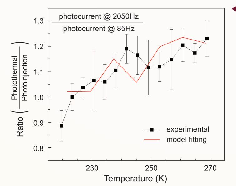
■ The photocurrent at 2050 Hz and 85 Hz represent the contributions from photoinjection and photothermal effects, respectively. The ratio increases with increasing temperature, indicating a larger photothermal compoenent at higher temperature.
