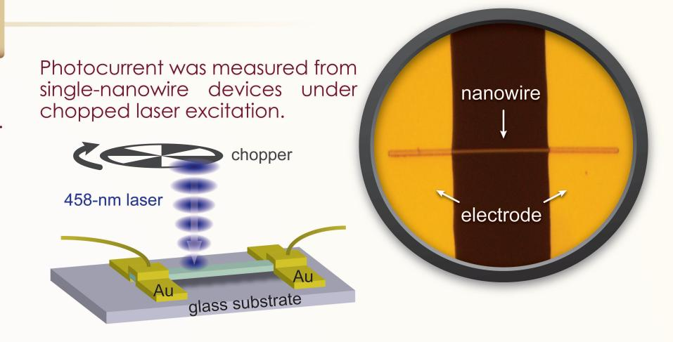
The slow photothermal response can be observed obviously in the waveform of the AC photocurrent with 200-Hz chopping frequency.
