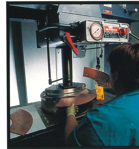
▲ Testing magnets' copper plates for consistency in strength and smoothness is the job of assembly technician Dianne Burns, shown here subjecting a plate to 95 tons of pressure per square inch.
